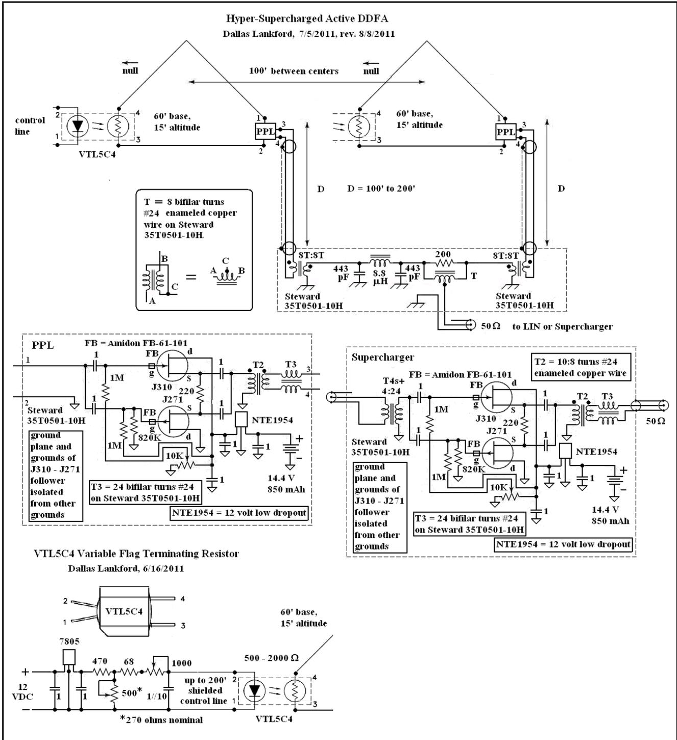
Originally, I developed a broadband 1x version of N4IS' high Q tuned LC front end 6x BF981 preamp and used it at the receiver end of the twin lead lead in, like he did. This led me to a different amplifier, a broadband low noise high intercept J310 - J271 FET follower, which was basically the "active part" of a simple, but very good, active whip antenna. Later, when I began investigating the broadband high performance FET follower connected directly to the antenna elements, the
